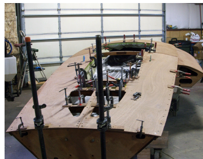
Ski installed with many c-clamps.
