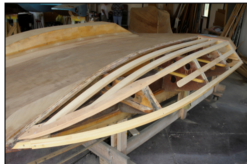
New battens installed in sponson bottoms.
