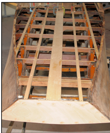
New keel, new bottom battens installed.
