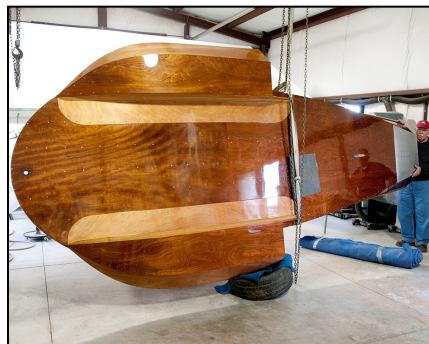
Completed bottom, ready to turn over.
