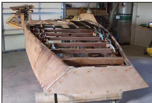
New frames, new transom, and covered sides of Helter Skelter .
