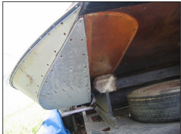
The aluminum cladding on the sponson was in place. Looks like there might be patch or modification on the bottom.
