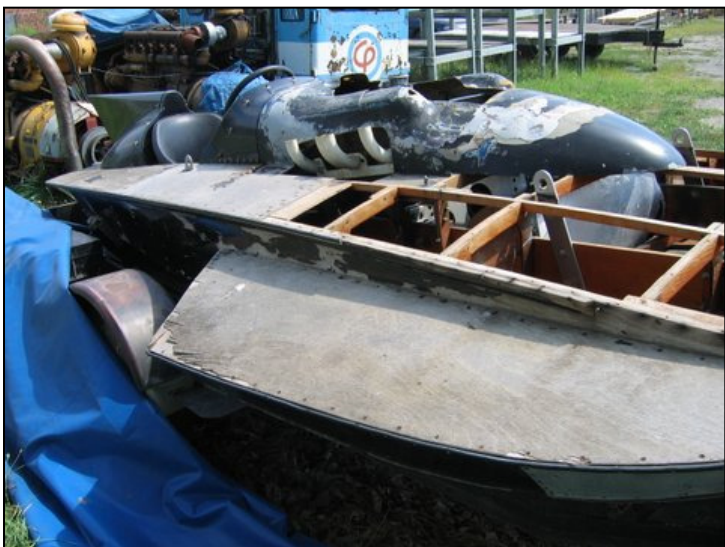
The cowling has been butchered and half the deck gone. Not the best of signs.
